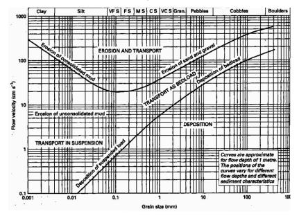
Figure 5.8 Hjulstrom Curve
