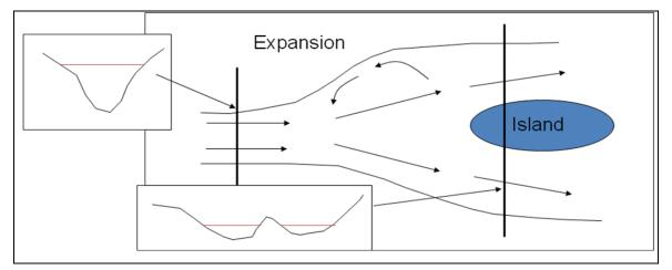
Figure 5.1 Schematic of 1D cross-section interpolation
