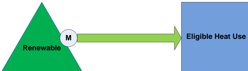
Figure 1: Under the new proposals if the external pipe is insulated a meter may only be required at the point of generation or the point of use.
