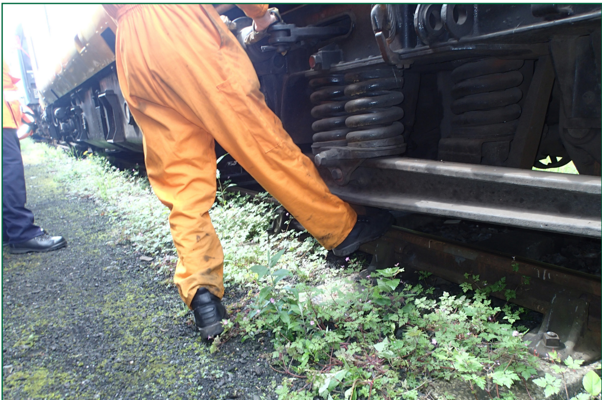
Figure 8: A post-incident reconstruction of how the scotch was driven against the wheel tread
