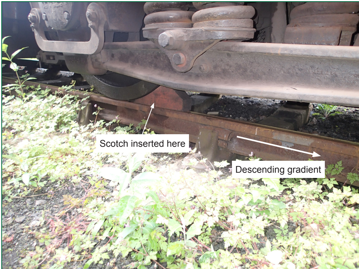
Figure 7: The position of the scotch as it was placed during a post-incident reconstruction
