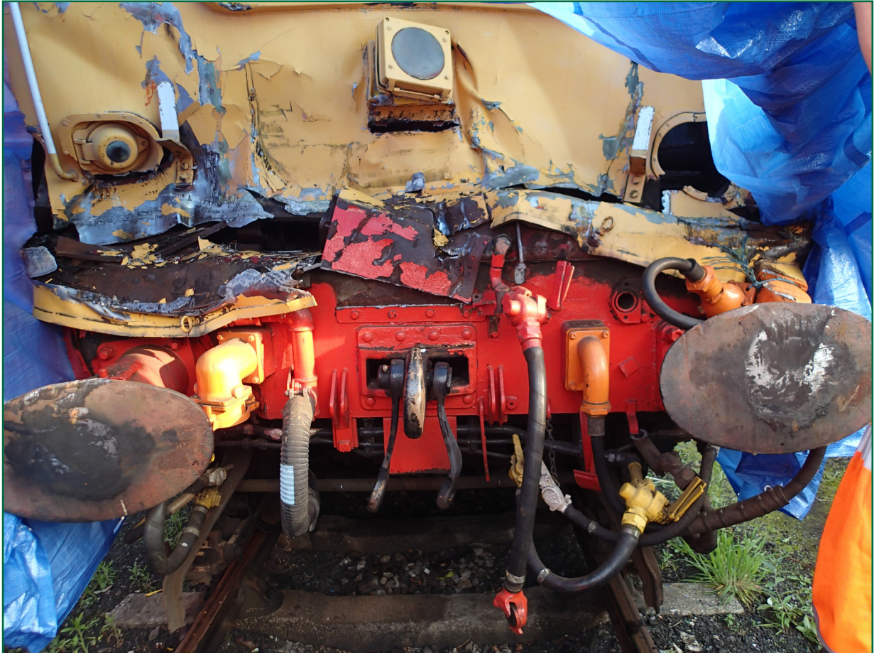
Figure 10: Damage sustained by locomotive 37198 following the collision
