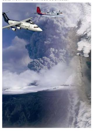
The Natural Environment Research Council's (NERC) Airborne Research and Survey Facility flew its Dornier 228 research aircraft in April 2010 to the edge of the volcanic plume over Britain caused by the Icelandic volcano Eyjafjallajökull, recording data relating to the height, density and position of the plume.
