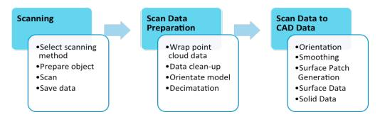
Figure 1: Workflow for scanning an object
