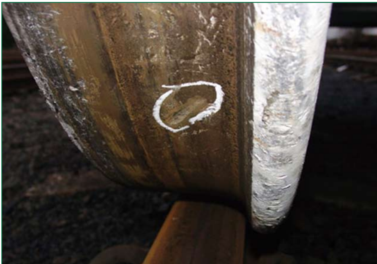
Figure 9: Damage to wheel three from number 788 points check rail
