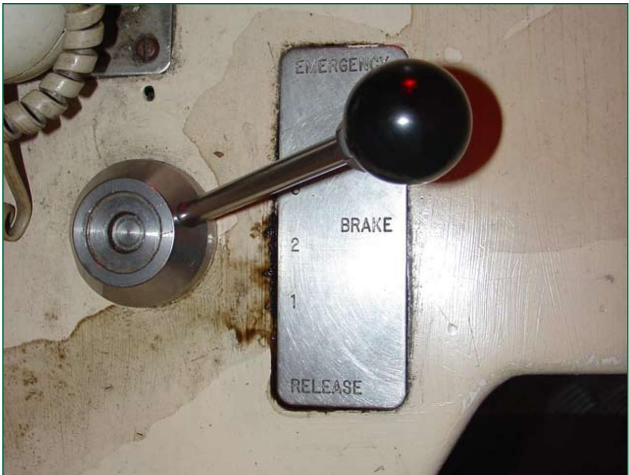
Figure 10: Brake control handle
