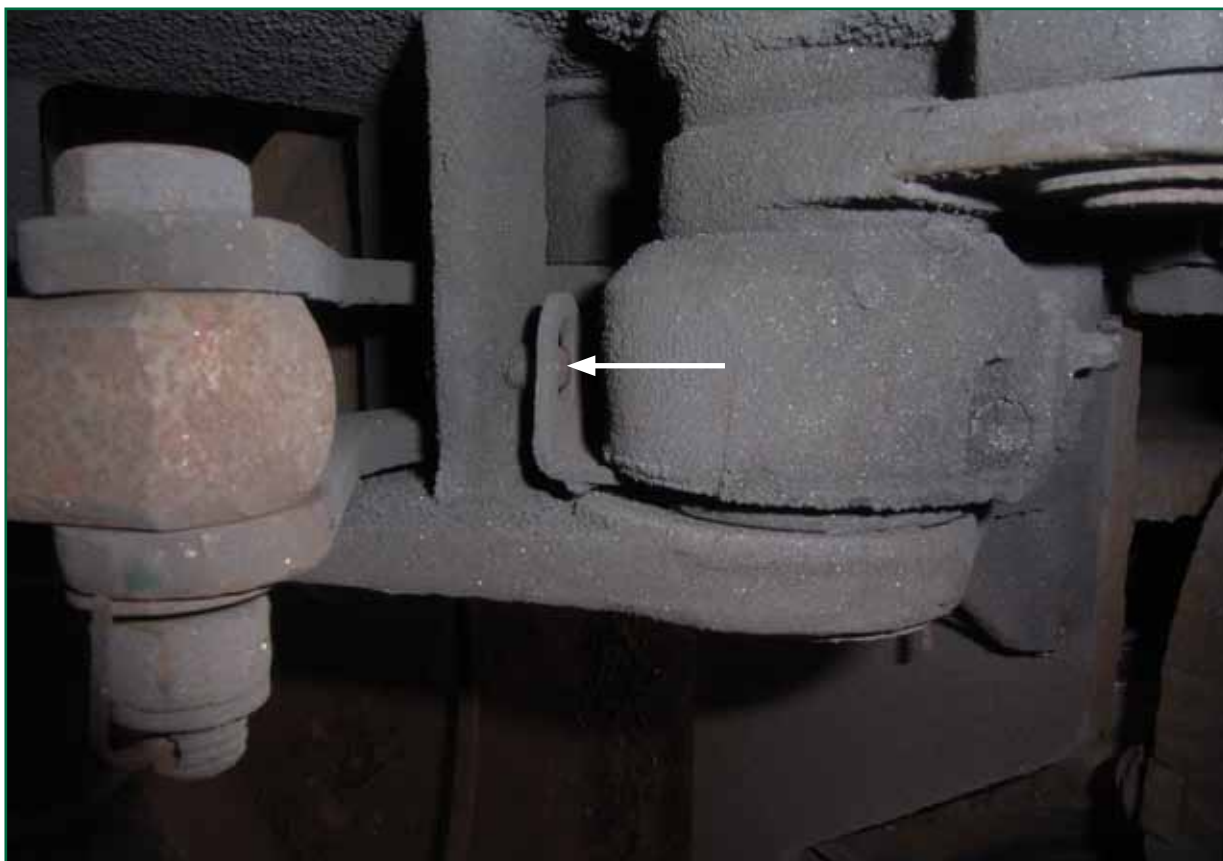
Figure 9: View of brake unit from below showing (arrowed) slack adjuster anchor bolt on VTG 3478
