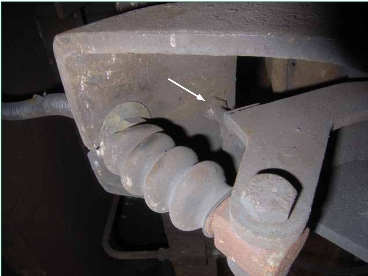
Figure 6: Handbrake cable and attachment to arm. Stop bolt (arrowed) in contact with bracket
