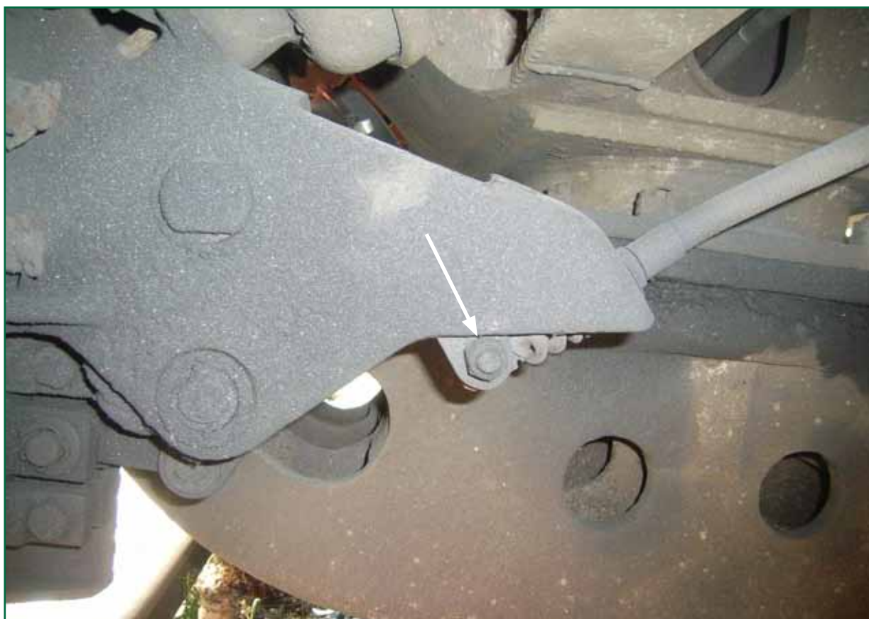
Figure 8: Brake unit on wagon VTG 3510 showing (arrowed) handbrake cable bolt fouling brake unit housing
