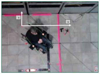
Figure F2: Tracked wheelchair (green lines) as it rolls down a 2° (1 in 28) slope
