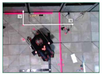
Figure F3: Tracked wheelchair (green lines) as it rolls down a 5° (1 in 11) slope
