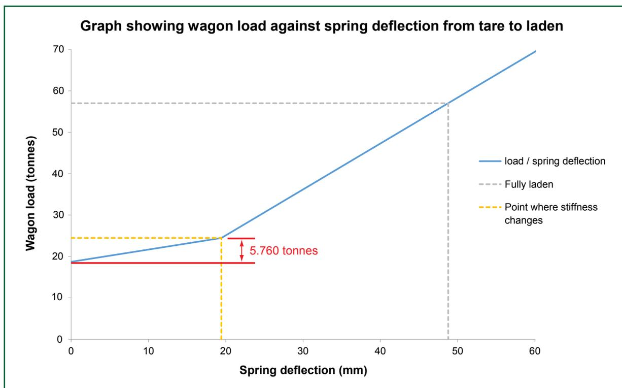
Figure 24: Wagon load versus spring deflection graph
