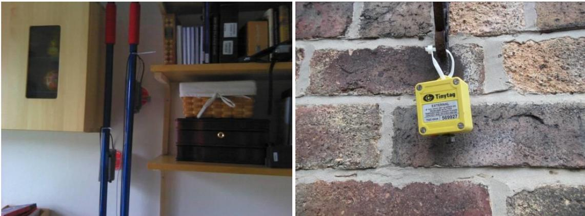
Figure 3 - The equipment installed in an occupied dwelling (left hand picture) showing the heat flux plates (red discs) and indoor temperature sensors supported by teleprops (blue poles) and clamps. Also shown is a Tinytag datalogger (right hand picture) attached to the outside wall (in a location out of direct sunlight)
