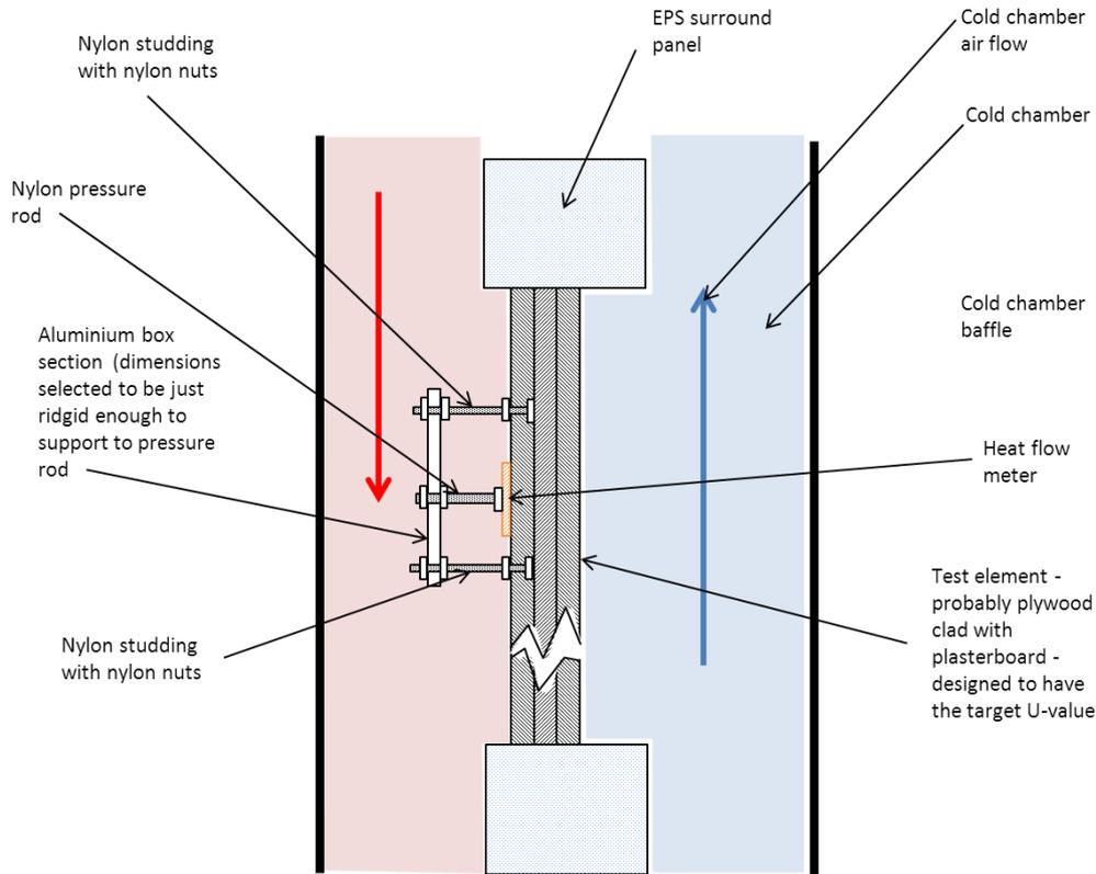
Arrangement for applying pressure to HFM to ensure it is in good contact with test element and to mimic method used in practice
