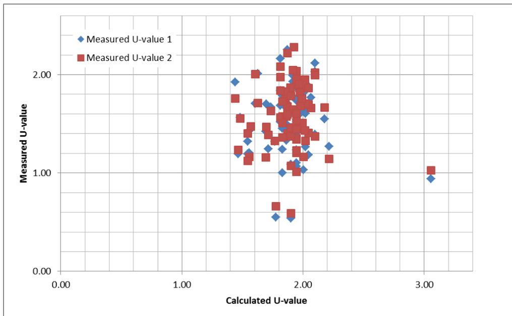
Figure C2: Scatterplot of measured against calculated U-values of standard solid walls using the final wall type classification and filtering data for low temperature differentials etc. Note that the majority of outliers visible in Group A of Figure C1 have now been reclassified as having been in insulated cavity walls.
