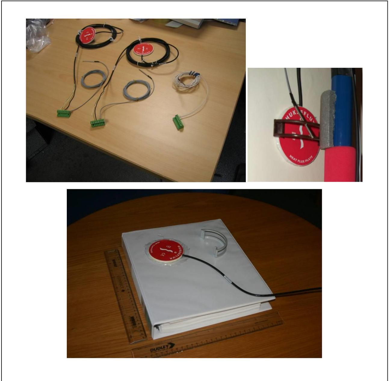
Figure 1 - The sensing equipment that was used for monitoring the heat flux and temperatures. The Hukseflux heat flux plates (circular plates) measure heat flux (in watts per square metre) and the thermistor sensors (silver tubes) measure temperature.
