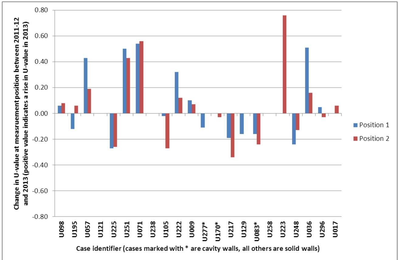
Figure 20 - Change in U-values between winter 2011-12 and 2013 at approximately equivalent positions.
