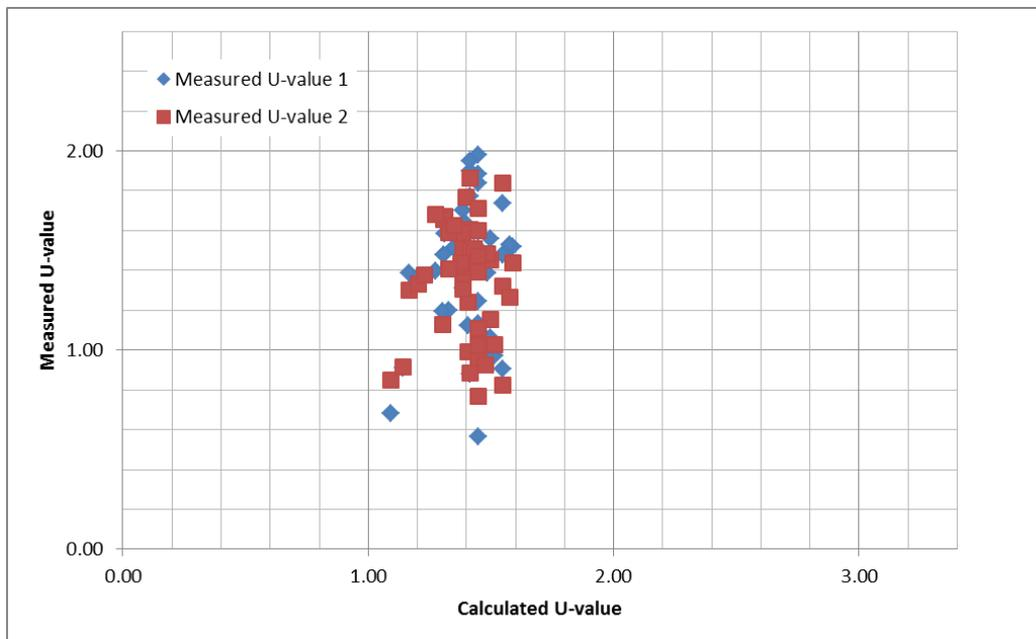
Figure C6: Scatterplot of measured against calculated U-values of un-insulated cavity walls using the final wall type classification and filtering data for low temperature differentials etc. Note the removal of several properties identified in group A of Figure C5 from this group.
