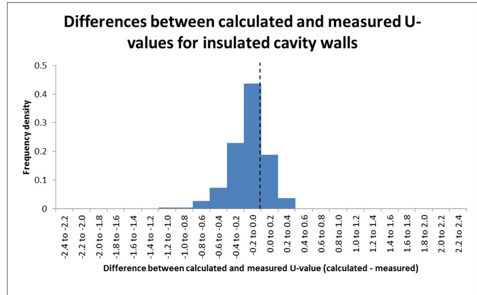
Figures 10 to 13: Frequency density distributions of differences between calculated and measured U-value for all measured points, for each type of wall measured. Dashed line shows position of zero difference.
