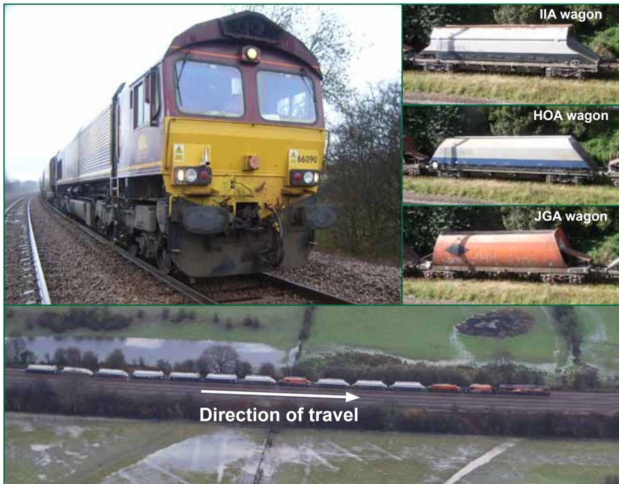
Figure 4: Class 66 locomotive (above left); IJA, HOA and JGA wagons (above right); and Train 6L73 (below - photograph courtesy of Network Rail)
