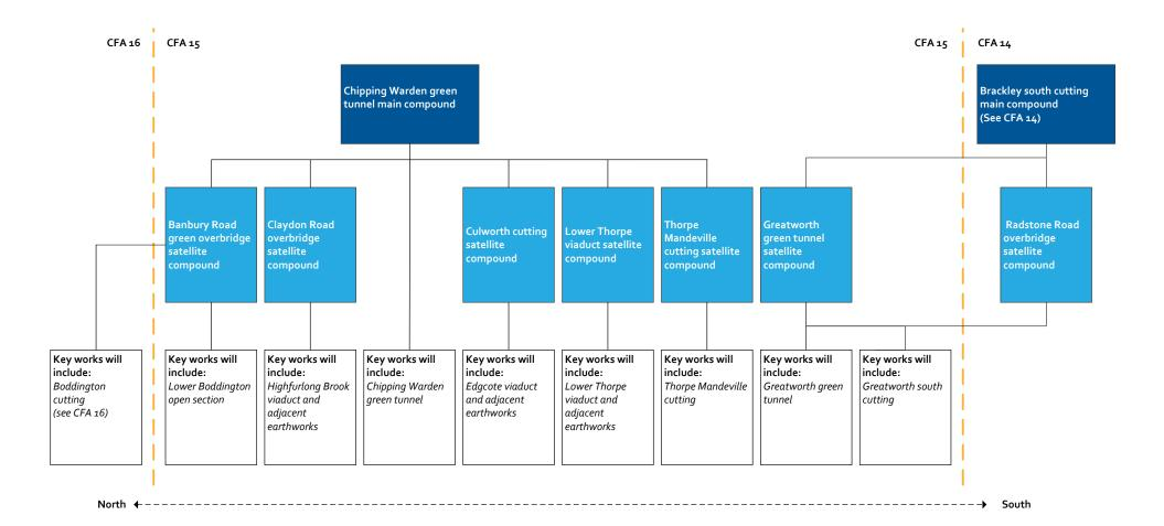
Figure 4: Schematic of construction compounds for railway installation works
