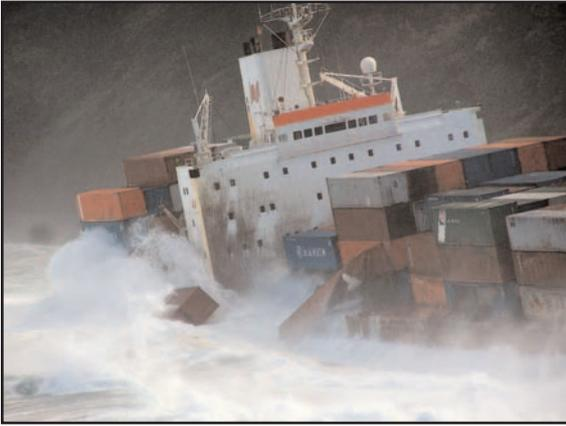
The 15,145gt Bermuda registered container vessel CP Valour, grounded in a bay off the NW coast of the island of Faial, Azores, on 9 December 2005. The next day, in worsening weather conditions, the vessel's hull began to fracture, causing substantial pollution. The subsequent salvage operation was unsuccessful and, about 3 weeks later, she was declared a constructive total loss and abandoned.
