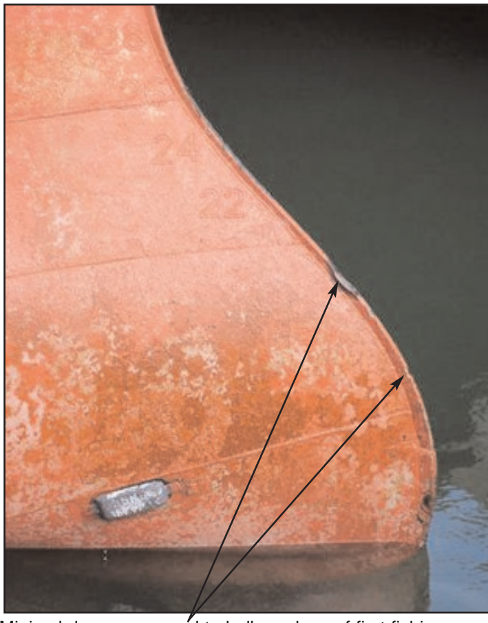
Minimal damage caused to bulbous bow of first fishing vessel
