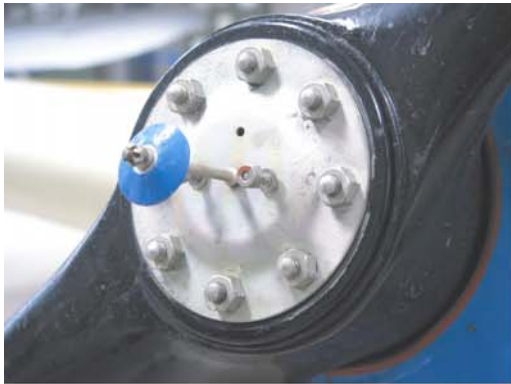
Figure 1a:- Right propeller installation (Spinner and lock plate removed) Note NO Belleville washers
