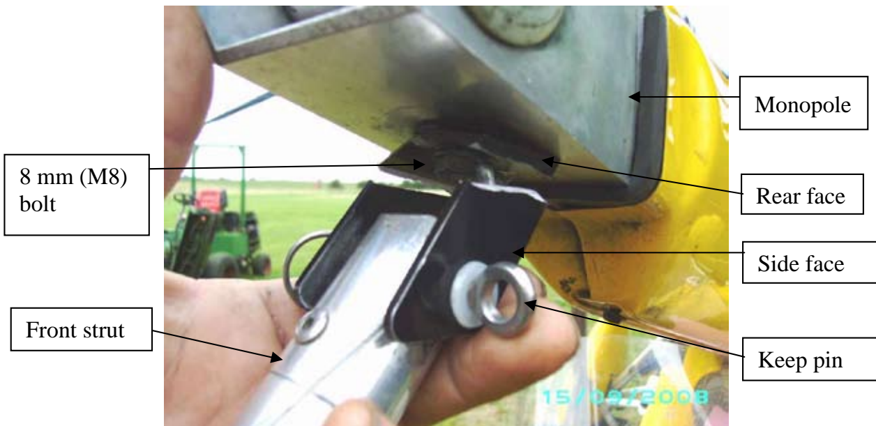
Figure 1 Failed front strut bracket on G-BZMI
