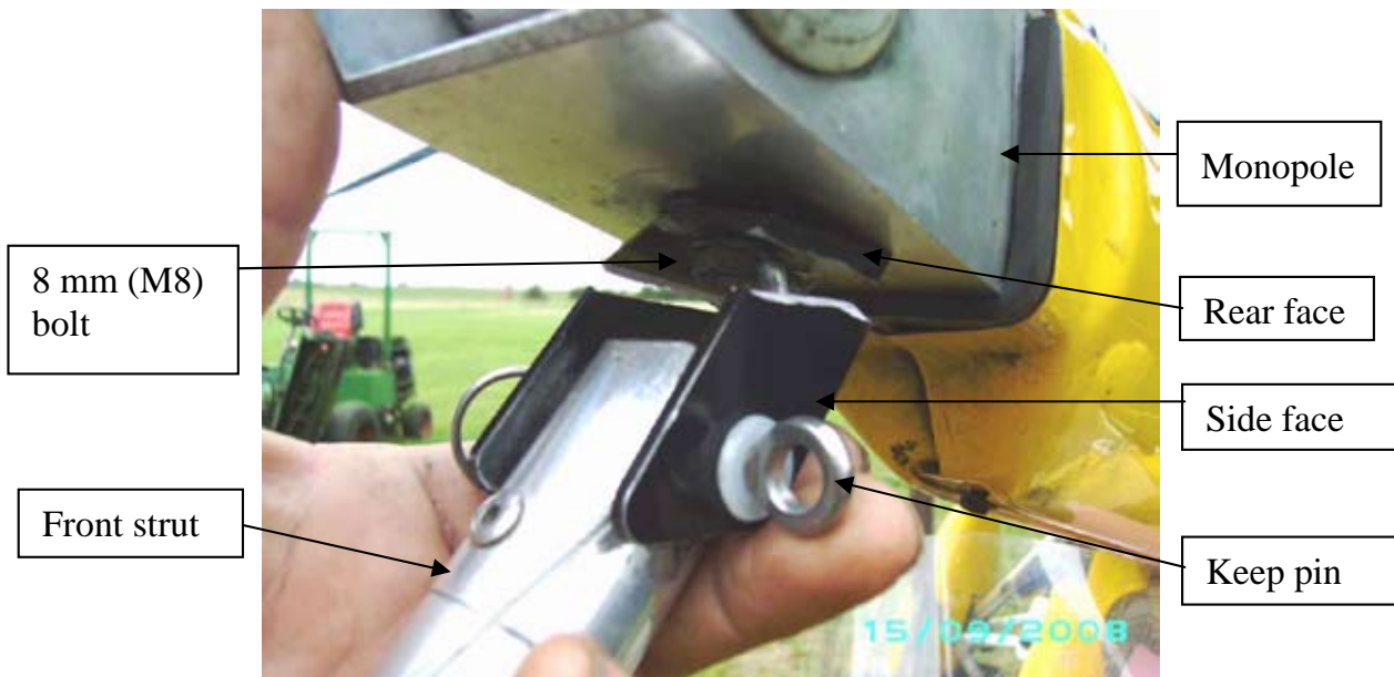
Figure 1 Failed front strut bracket on G-BZMI
