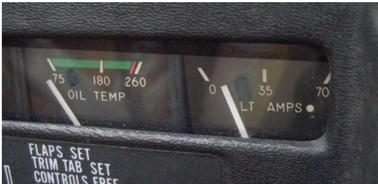
Figure 2 Ammeter zero error of approximately 10 amps
