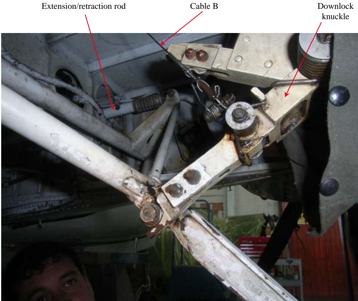
Figure 1 Gear down and locked
