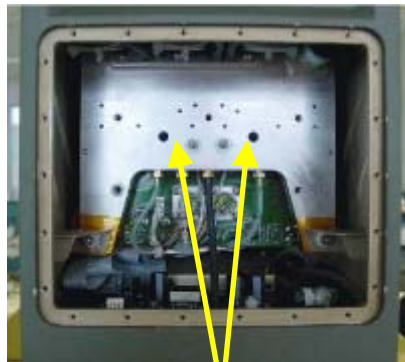
Wipe the air inlet ports
