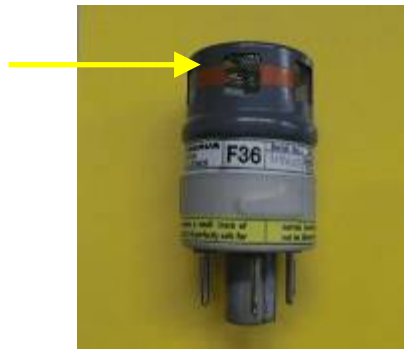
F36 Smoke Detector
