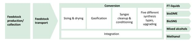
Figure 3: Generic process schematic for gasification with five catalytic synthesis types
