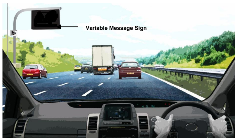
Figure 4B: Illustrative M1 junction 19 to 16 smart motorway all lane running scheme section operating in normal motorway conditions with a blank verge mounted variable message sign
