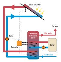
Figure 1 Typical twin coil solar thermal system
