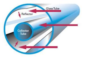
Figure 8 Schematic of heat pipe evacuated tube collector
