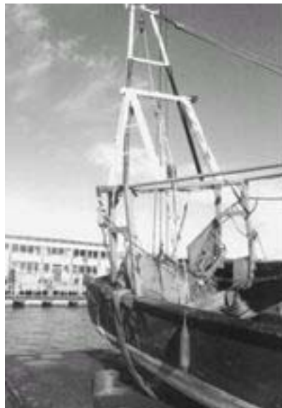
The gantry and A frame
