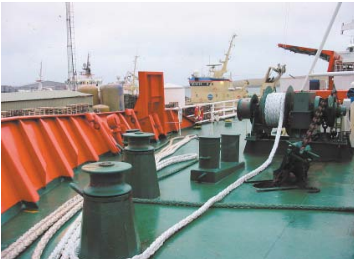
Polypropylene rope flaked out for use as a spring
