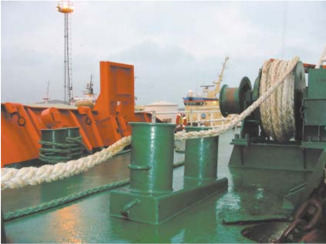
Rope led between the bitts on the starboard side
