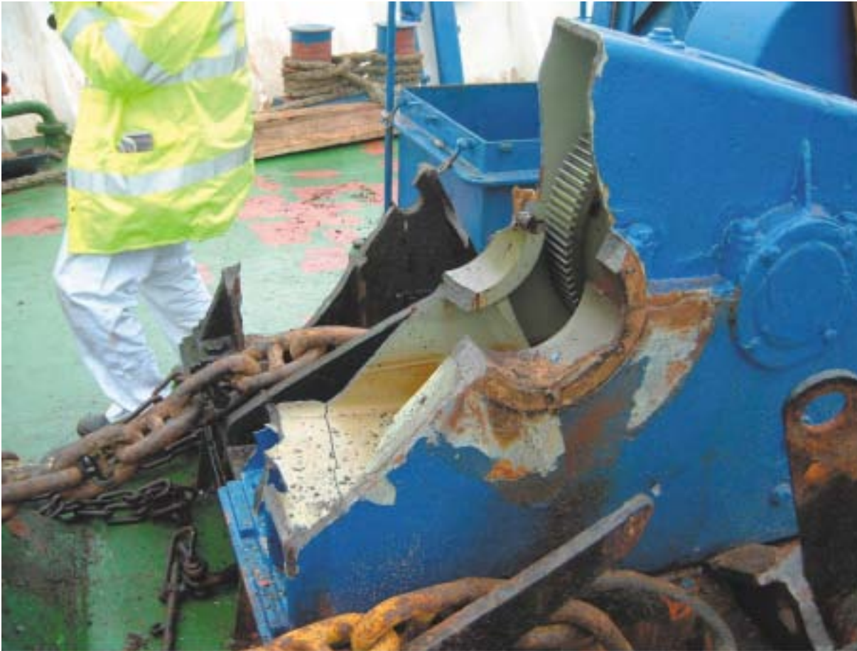
Windlass after catastrophic failure
