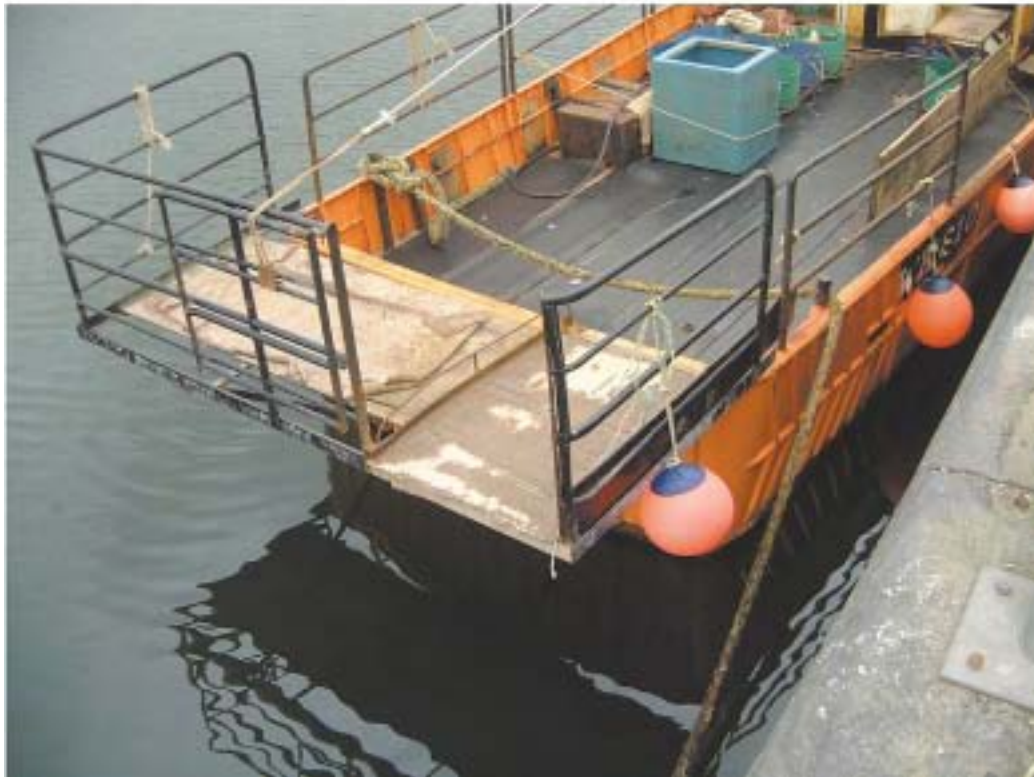
Working deck area showing pound board arrangement
