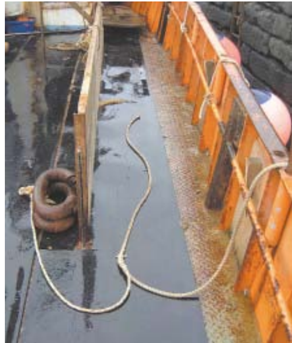
Working deck area showing configuration of back line
