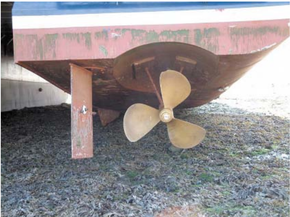
Photographs of hull showing position of propeller and offset rudder
