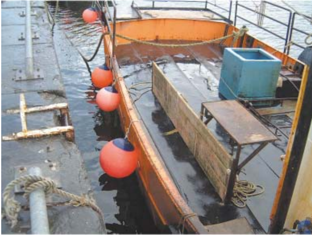
Working deck area showing pound board arrangement
