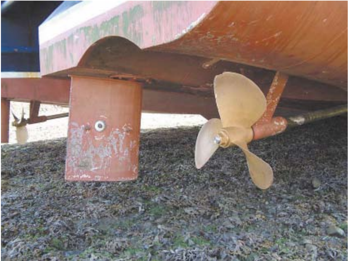
Photographs of hull showing position of propeller and offset rudder
