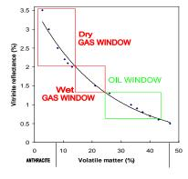
Fig. 9 Hydrocarbon maturity windows and main coal maturity indices. The oil window ranges from 25-43% volatile matter, and the wet gas window ranges from 14-25% volatile matter.
