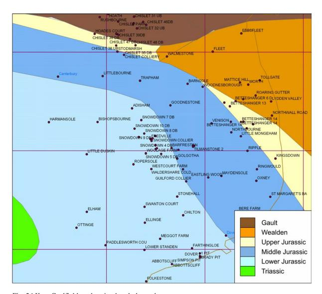
Fig. 26 Kent Coalfield exploration boreholes and supercrop
