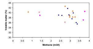
Fig. 12 Methane content plotted against percentage volatile matter (analyses of coals at approximately the same depths).
