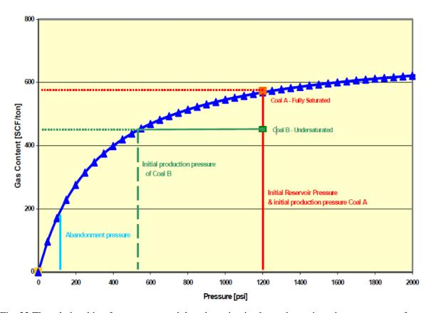
Fig. 22 The relationship of gas content and the adsorption isotherm determines the gas recovery factor
