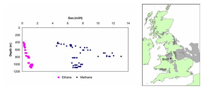
Fig. 5 Methane and ethane content in the Birch borehole, as measured and recorded in the National Coal Board database. Coals below 800 m have lower than expected methane contents (about 4m³/t lower), which are partially offset by the more rapid increase in ethane content below this depth.
