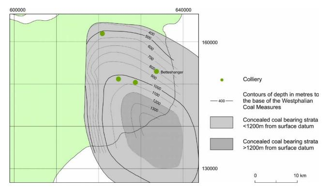
Fig. 25 Kent Coalfield mines and depth in metres to the base of the Westphalian Coal Measures. Note that no part of the Kent Coalfield is considered to have 'good' coalbed methane potential based on the low NCB gas contents (but see discussion in text and Fig. 7).
