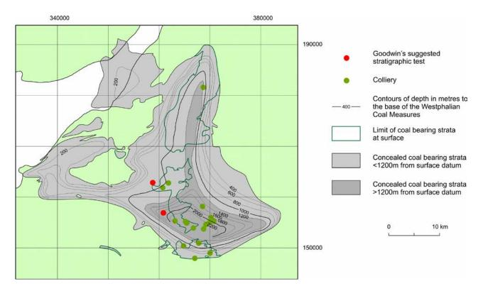
Fig. 35 Contours of depth to the base of the Westphalian Coal Measures in the Bristol-Somerset Coalfield.
