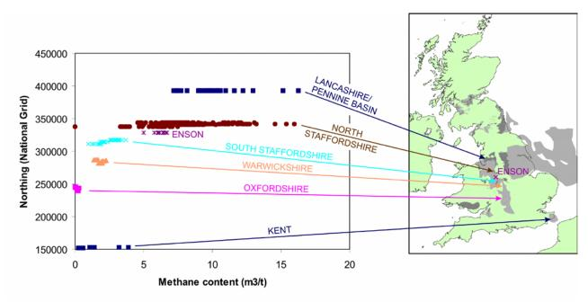
Fig.7 Northward increase in Methane content in coals by coalfield. The range of gas contents is shown. Enson is a borehole on the Mesozoic ridge between the South and North Staffordshire coalfields. Kent and South Wales (not shown) coalfields in the Variscan foredeep have higher values than those of the foreland but Kent's are lower than would be expected from their maturity.
