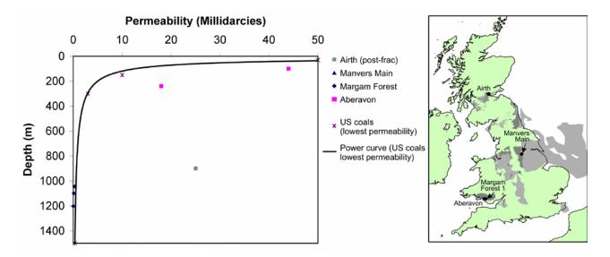
Fig. 16 A plot of UK coal permeability and the lowest permeability values of US coals vs. depth.
