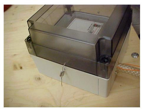
Figure 2 Pressure Sense Switch with Security Seal
