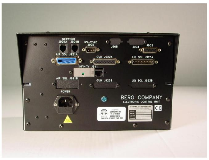
Figure 7 Infinity Electronic Control Unit (ECU)
