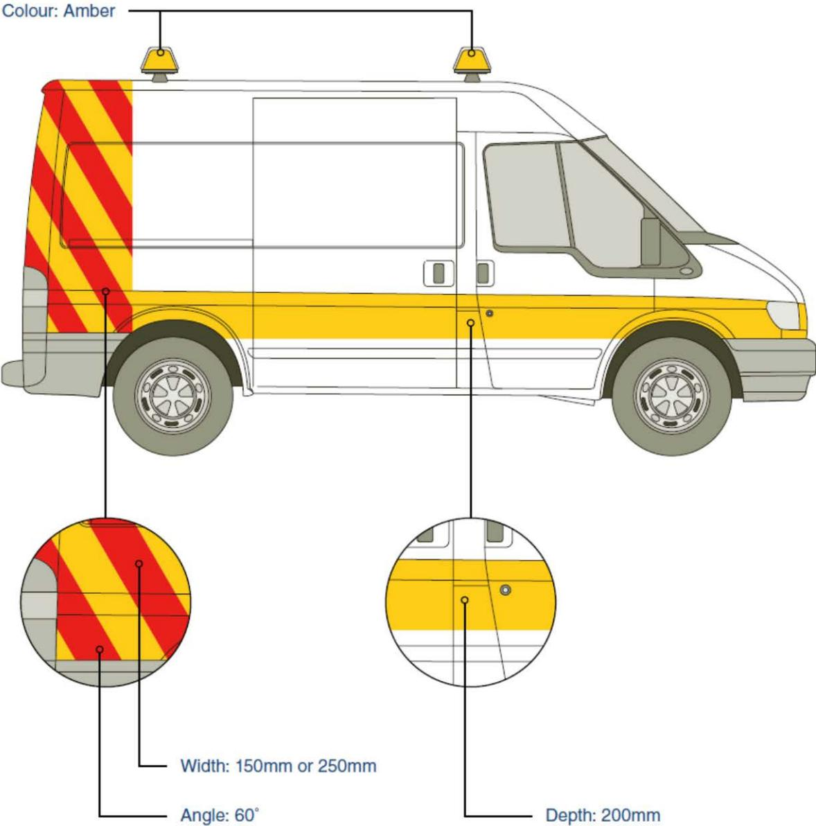
Figure 2 – Illustration of an escort vehicle (not to scale)
