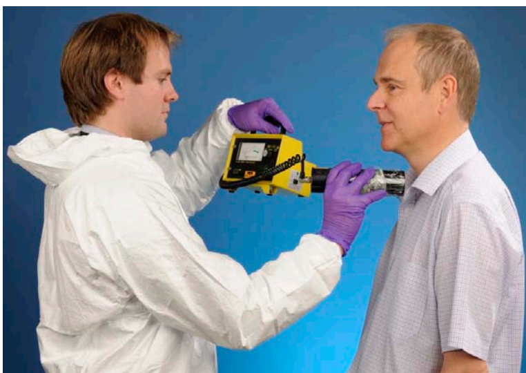
Figure C4 Monitoring of the thyroid for I-131 with a hand-held radiation monitor
