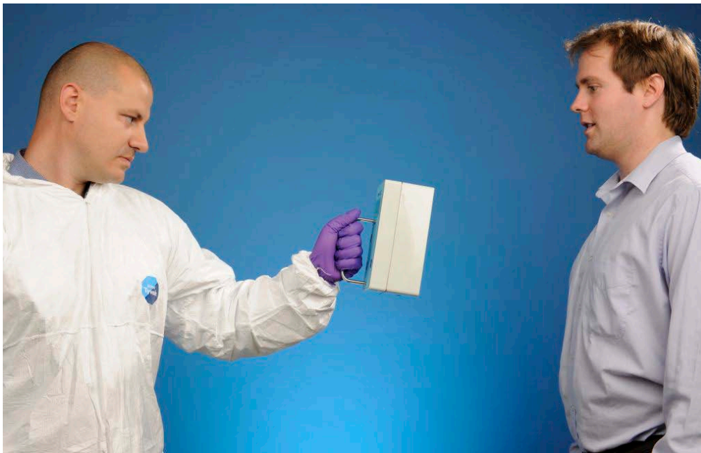
Figure C1 Monitoring of whole body activity with a hand-held radiation monitor
