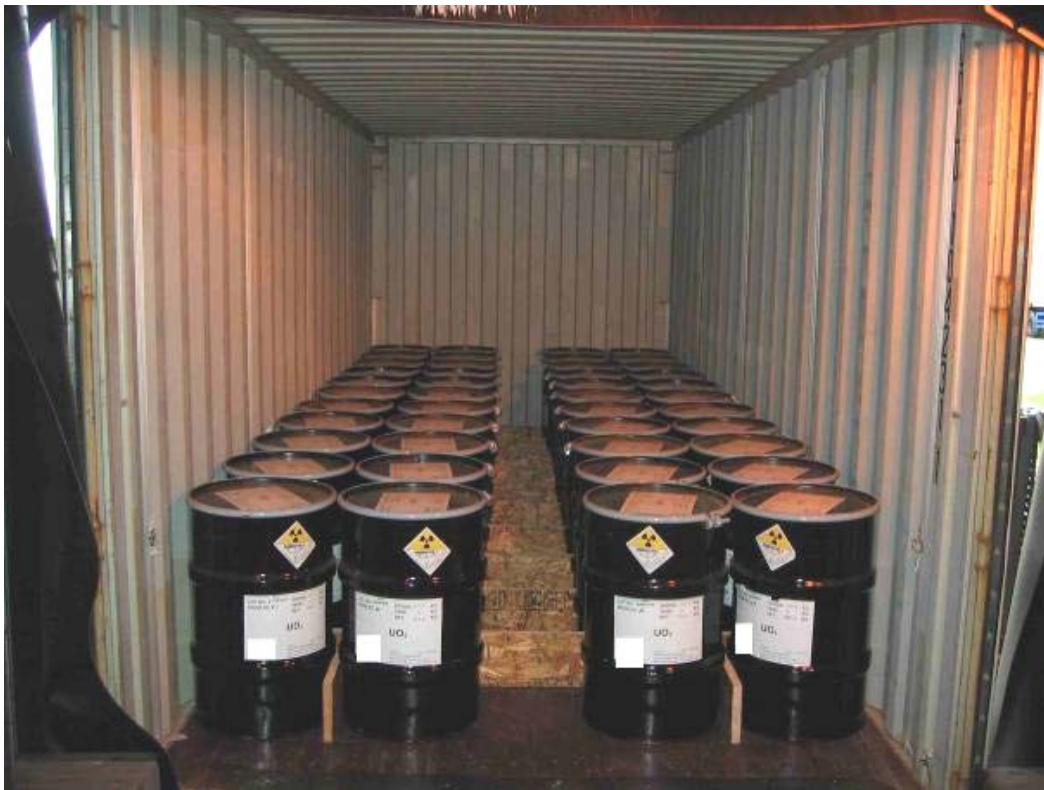
Figure 2. Drums of UO 3 inside a freight container
