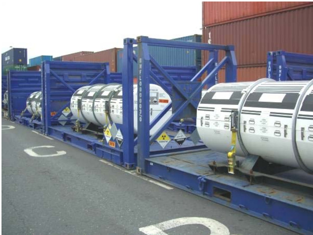
Figure 6. Natural UF 6 in 48Y cylinders fixed within flatracks in a dockside storage area
