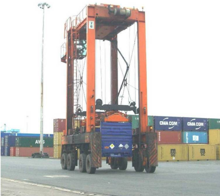
Figure 5. Transport of flatracks and containers in a port area by straddle carrier
