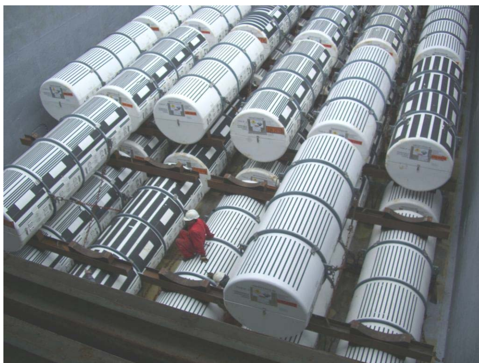
Figure 9. Fixing cylinders of depleted UF 6 in the hold with steel supports and lashings
