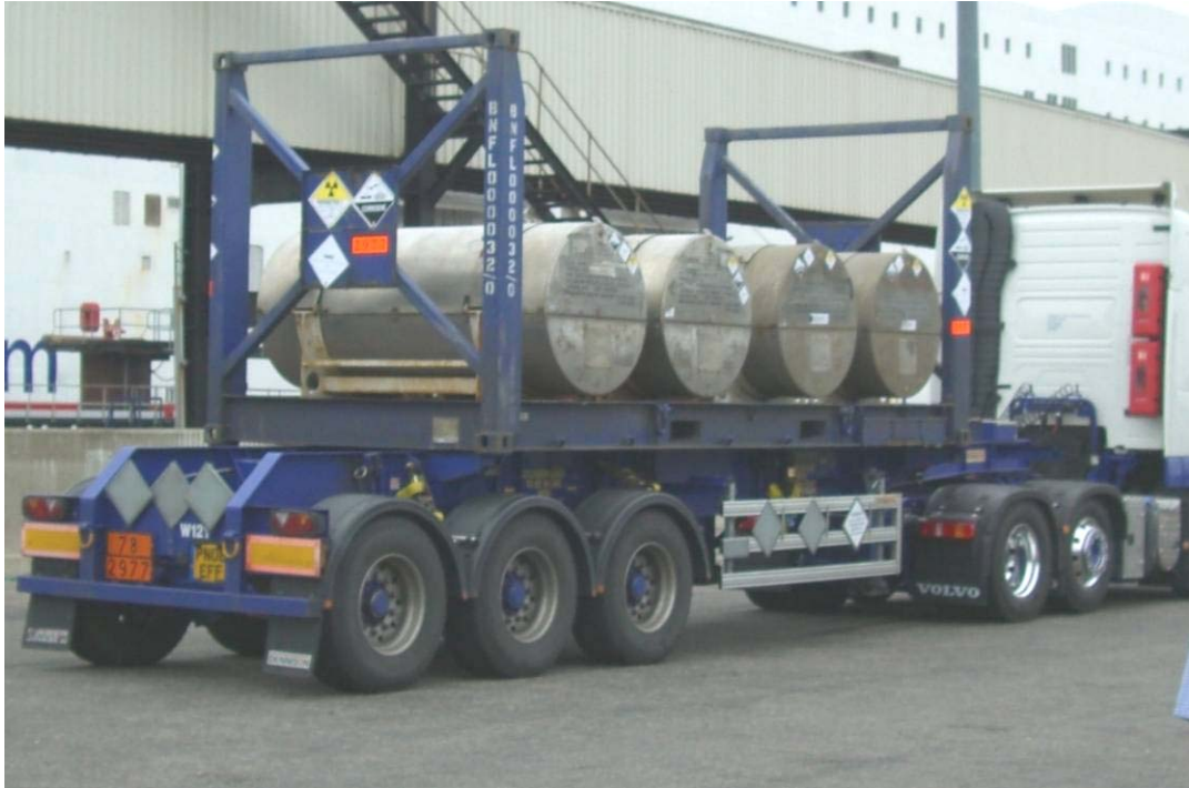
Figure 7. Four 30B cylinders containing enriched UF 6 fixed within a flatrack
