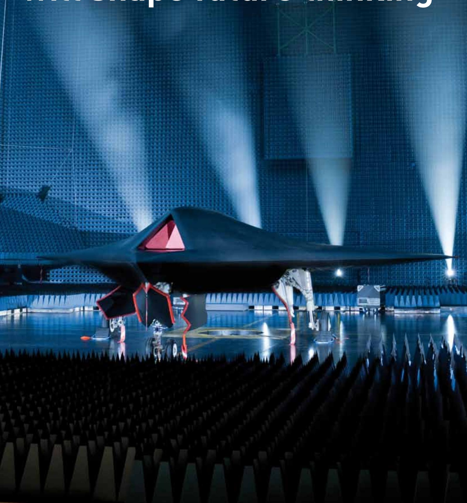
An unmanned combat aircraft of the future – Taranis – has been unveiled. Named after the Celtic god of thunder, the 12m long concept demonstrator with a wing span of 10m will test the possibility of developing the first ever autonomous stealthy Unmanned Combat Air Vehicle which would ultimately be capable of precisely striking targets at long range, even in another continent.
