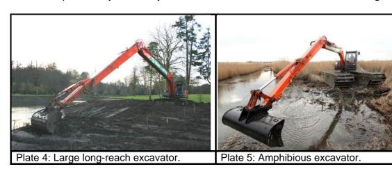
Two distinct construction methods will be used to restore the profile of the banks with the dredged material:
