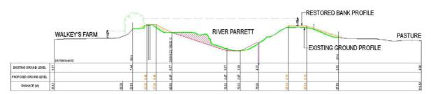
Figure 7.1 (not to scale): cross section through River Parrett showing the existing and restored bank profiles. A property on West Yeo Road (receptor R7) can be seen on the left. The Macmillan Way West (receptor R2) runs along the right embankment crest.
