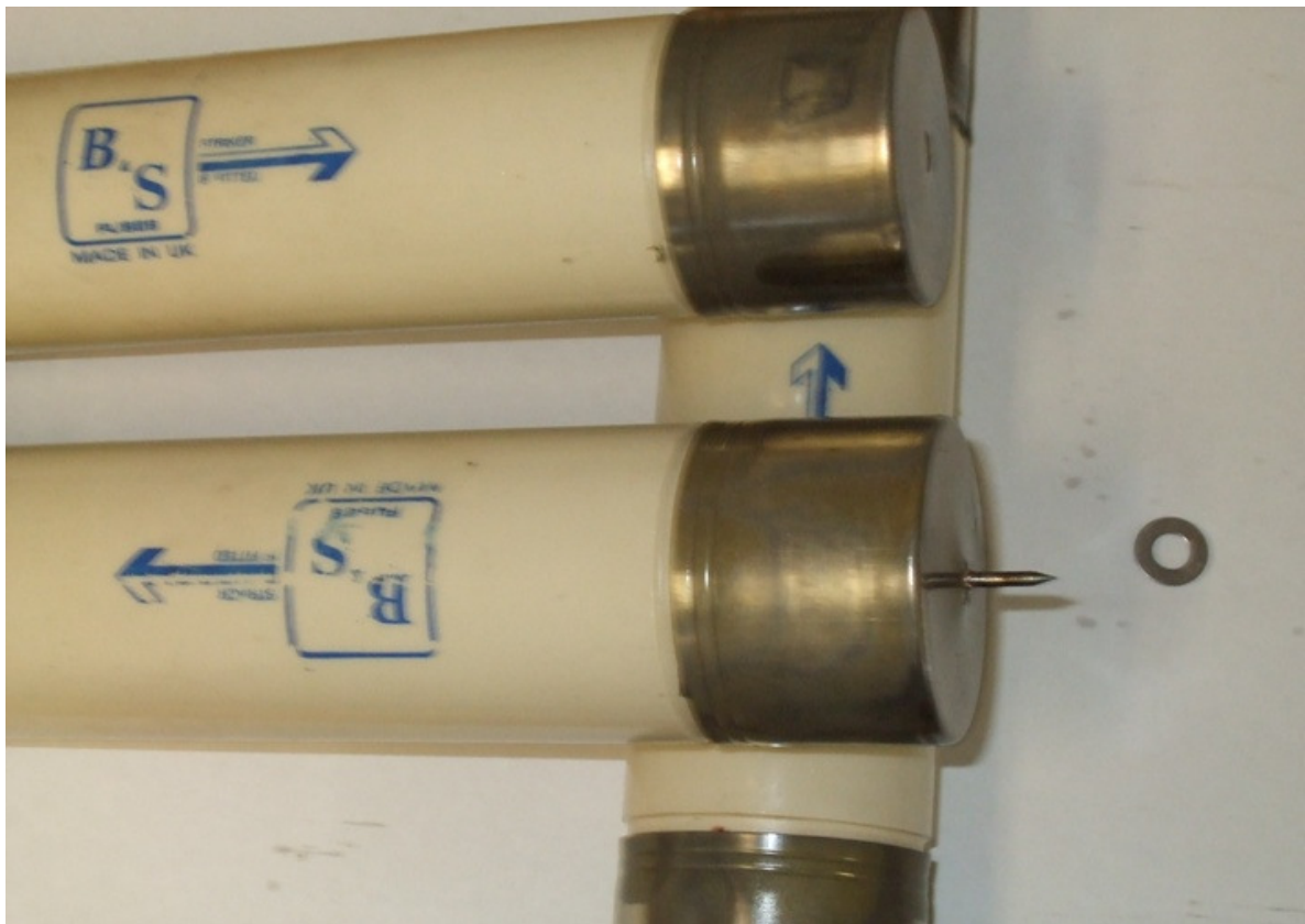
Photograph showing striker pin ejection in opposite direction to that indicated on fuse body.
