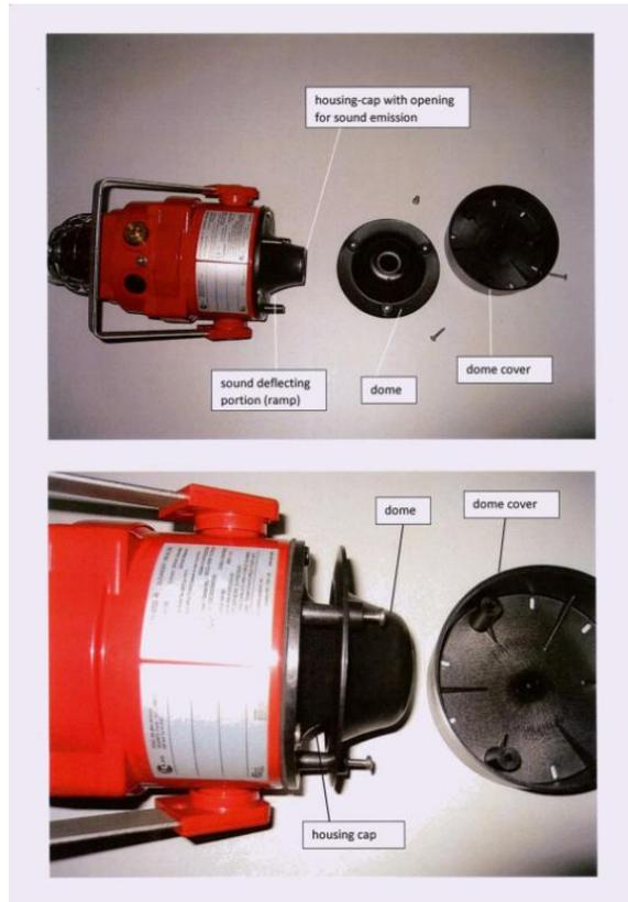
28. Therefore the Radial Horn alarm includes a dome mounted on top of the housing; the dome is arranged to emit sound from the audible alarm (i.e. the sound is emitted when it leaves the base of the dome); and the sound is emitted downwardly towards the housing (i.e. through the gap between the dome and the housing). Therefore it is my view that the Radial Horn alarm exhibits all the features of claim 1.
