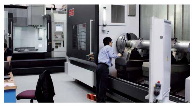
The High Value Manufacturing Catapult Centre includes the Advanced Manufacturing Research Centre (AMRC), University of Sheffield. This illustrates machining an engine rotor on a Mori Seiki CNC mill-turn machine at the AMRC's Rolls-Royce Factory of the Future.
