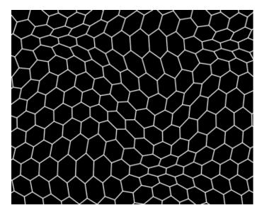
Representation of Graphene under strain.
