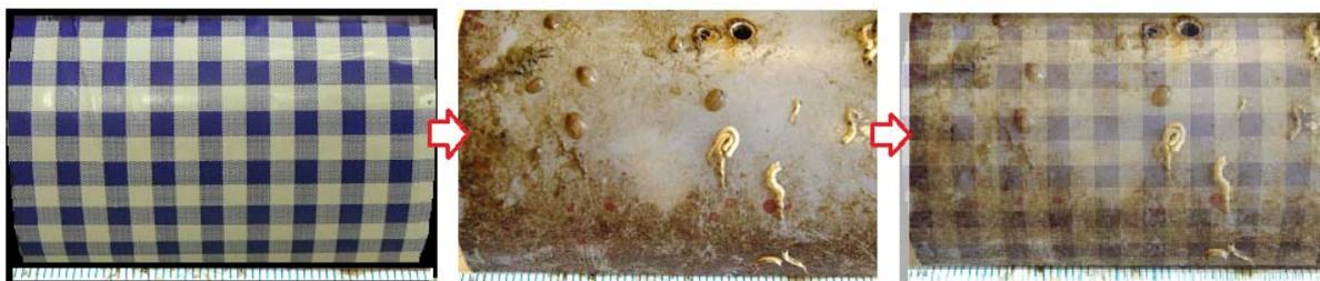
Figure 3. An example of quantifying colonisation using photographic overlaying
