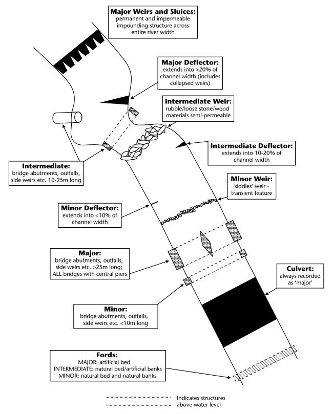
**Intermediate**: road or rail bridges **without any in-river supports**, and with bank abutments occupying 10-25m of the bank. **1** D3c.
