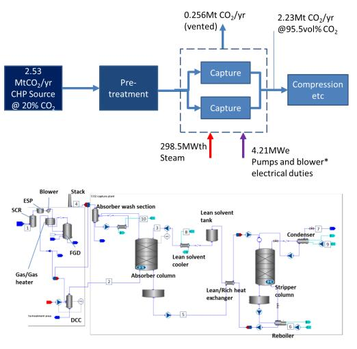
SCR – Selective Catalytic Reduction ESP – Electrostatic Precipitator FGD – Flue Gas Desulphurization DCC – Direct Contact Cooler
