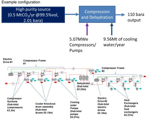
Figure 18 Overall schematic (Upper panel) and process diagram (lower panel) for multi-stage  $CO_2$  compression from 2 bara to 110 bara at a high purity  $0.5MtCO_2/yr$  source (see Appendix for details)
