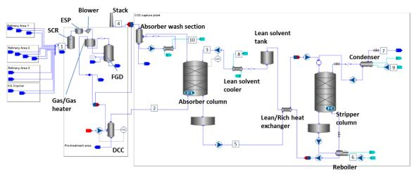
SCR – Selective Catalytic Reduction ESP – Electrostatic Precipitator FGD – Flue Gas Desulphurization DCC – Direct Contact Cooler
