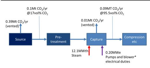
Figure 22 Illustrative schematic for 0.1 Mt/yr capture pilot using 1st generation amines at a cement plant in 2020.
