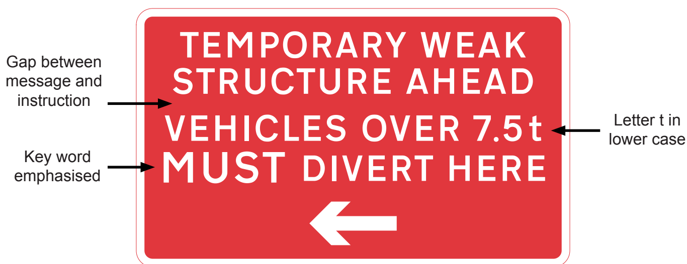
Figure 1 Example of a sign that can be created under regulation 53 showing several of the basic design features mentioned above.
