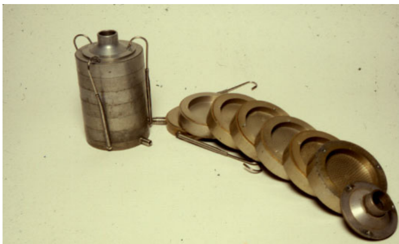
Figure 3.4 Andersen sampler showing six stages
