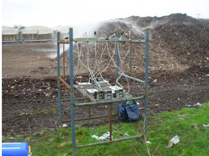
Figure 2.1 The two types of samplers with the pumps and sampling boxes on the lower platform for easy access, and the sampling heads at the end of the tygon tubing at a height of 1.8 m. The compost windrow can be seen in the background.
