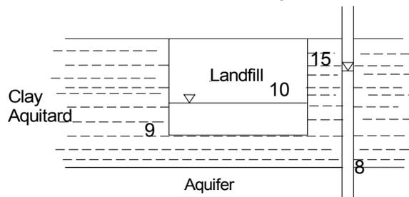
**Scenario 2:** A landfill with a geological barrier and an artificial lining system (including a geomembrane) in a permeable formation
