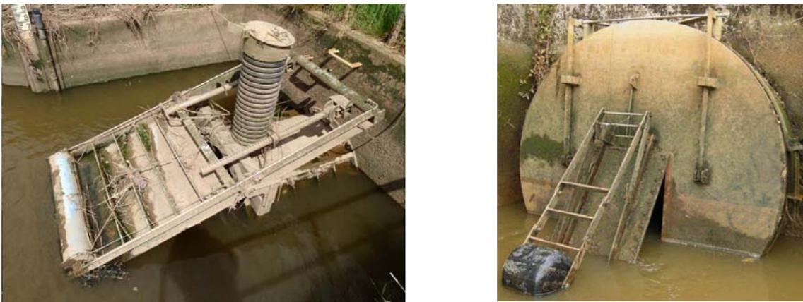
**Figure 1-1 Two examples of SRT designed overseas. Note floats have been removed from arms in first example.**
