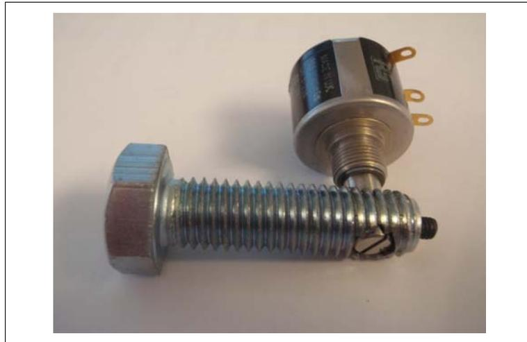
**Figure A2 Pendulum mounted on potentiometer**
