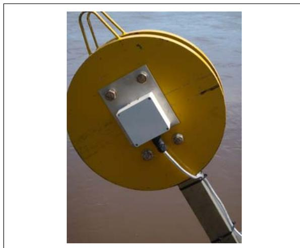
**Figure A3 Sensor mounting**
