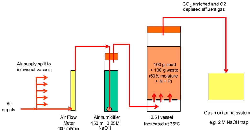
**Figure A3 Schematic diagram of aerobic DR4 test set up**
