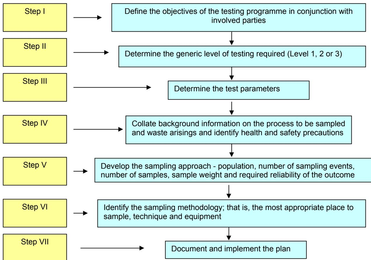
**Figure 5.2 Key steps in developing a sampling plan.**
