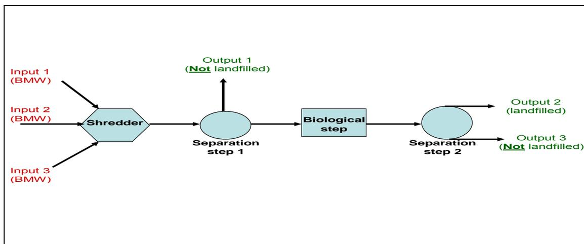
**Figure 8.1 Schematic of MBT plant where all three inputs are derived from municipal waste.**
