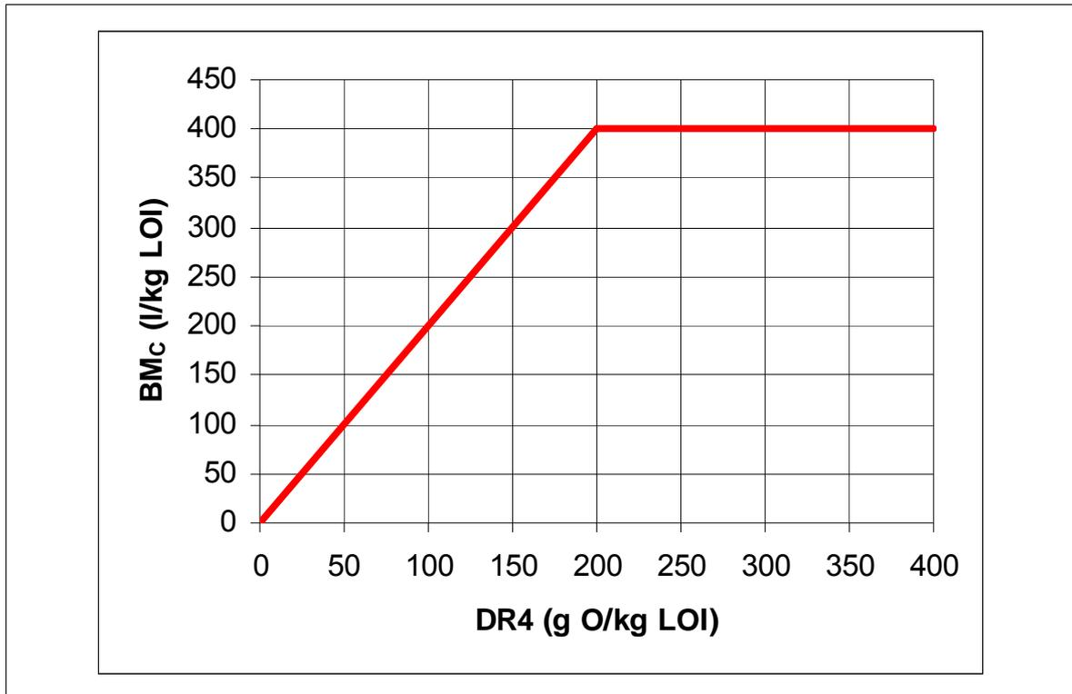
**Figure B.1 Default correlation between the aerobic DR4 and anaerobic BMc biodegradability tests.**
