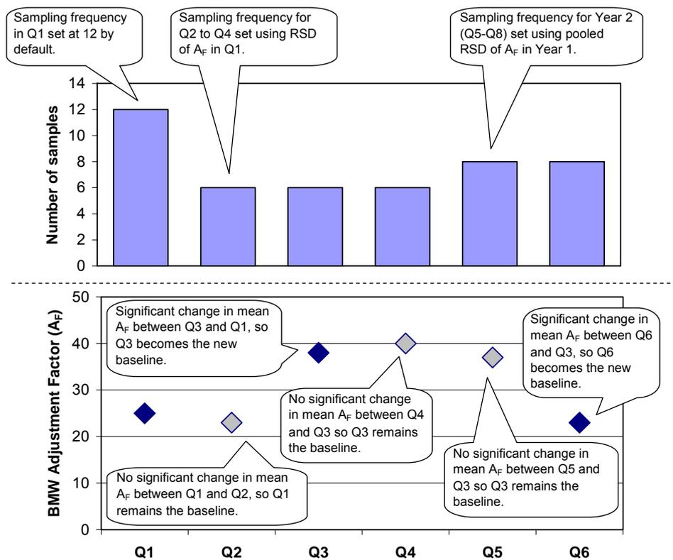
**Figure 6.3** Example showing how to determine the required sampling frequency and assess the performance of the plant using change in  $A_f$ .
