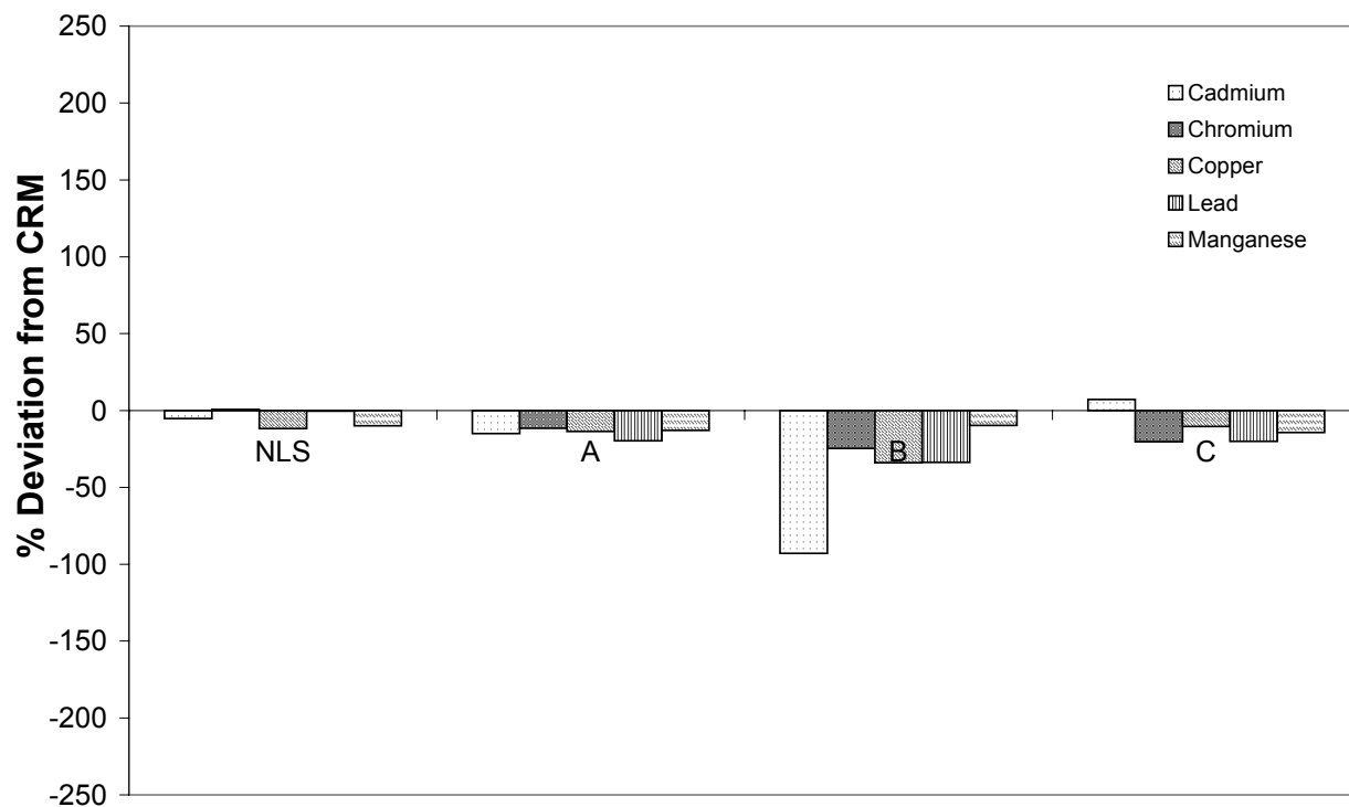
Figure 5.1 Comparison of laboratory performance for analysis of metals CRM (Cd, Cr, Cu, Mn and Pb)
