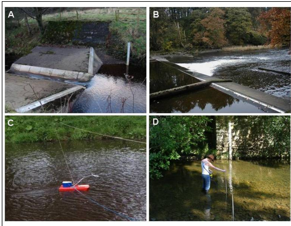
Figure 2. Instream methods of measuring flow-rate
