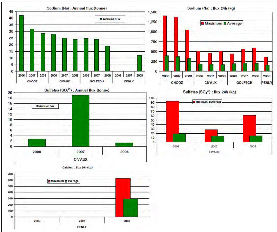
Figure A6.9 Sodium, sulphates and calcium discharges from demineralisation plants
