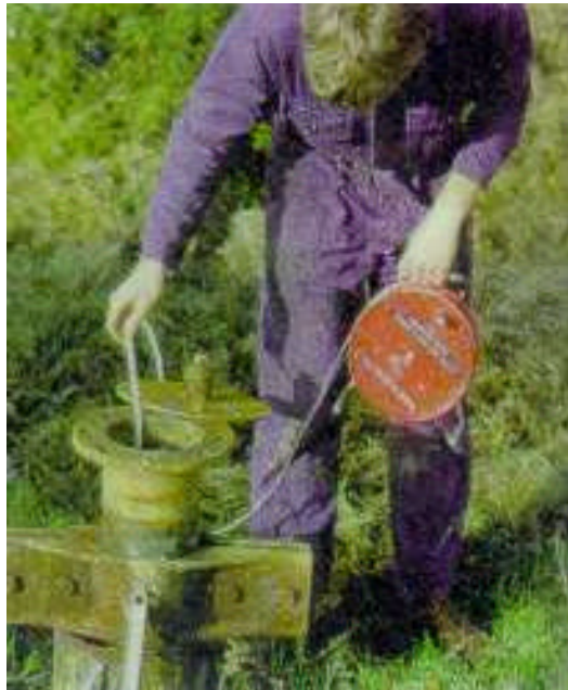
*Agency officer checking the groundwater level within a borehole
