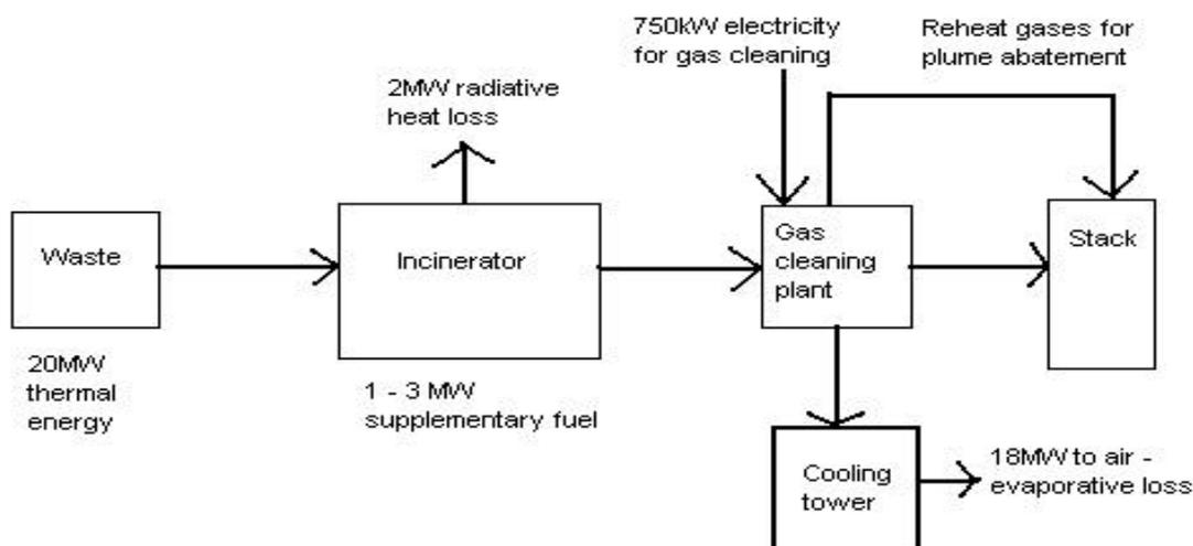
**Figure 9 Energy flows within a hazardous waste incinerator (Source: Shanks 2001)**
