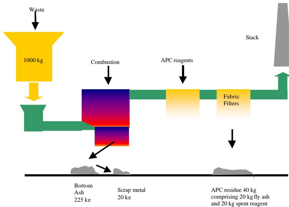
**Figure 4 Waste residue streams in a typical UK mass burn EfW combustion facility**
