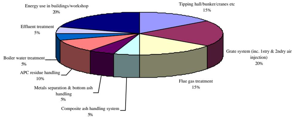
**Figure 7 Estimated distribution of energy consumption in a mass burn MSW incineration facility (Source: Courtesy of ONYX UK Ltd)**
