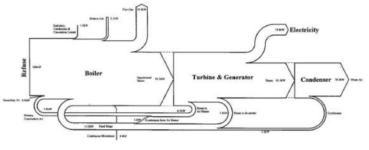
**Figure 8 Energy flows of a model waste to energy facility**
