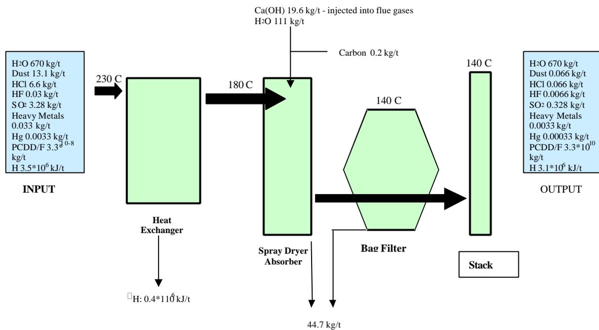
**Figure 1 Schematic of inputs and outputs for semi-dry abatement plant**
