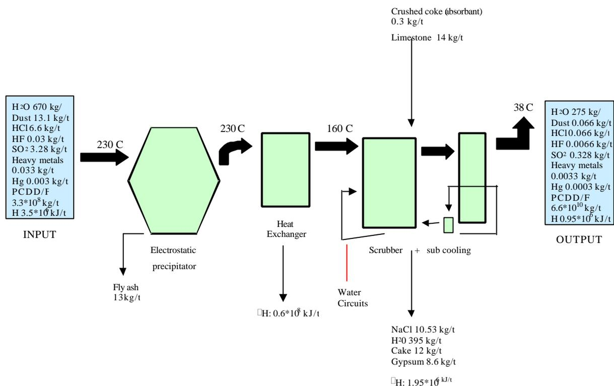
**Figure 2 Schematic showing inputs and outputs from wet scrubbing abatement plant**
